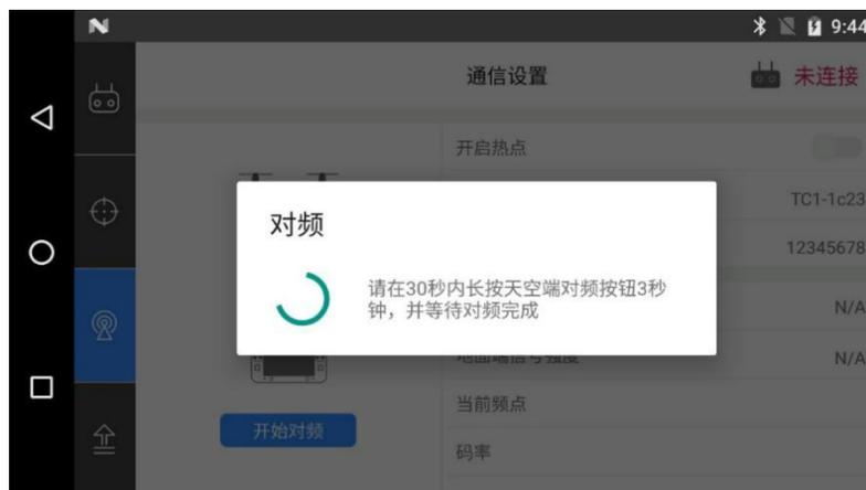
3. Use a sharp tool (e.g. a pen, etc.) to press the receiver's Frequency Matching button for 3s and release it to complete the frequency matching. After successful matching, the remote control indicator will be solid green. If the frequency matching button is not pressed within 30 seconds, "Frequency Matching failed" will be displayed.
