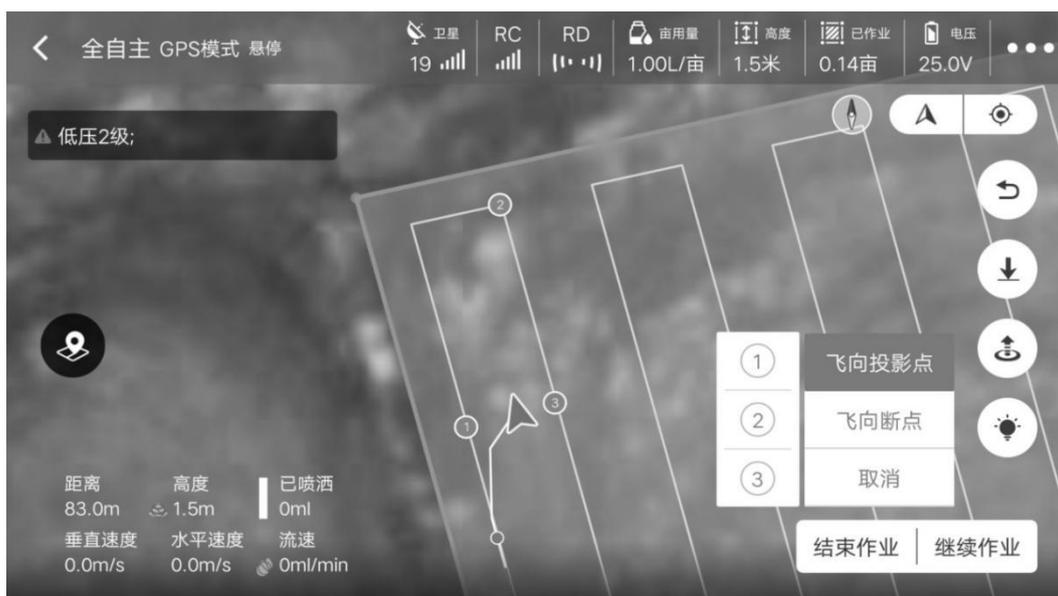
Step3. Click on one of the points, and the drone will fly to the point to continue the operation.
