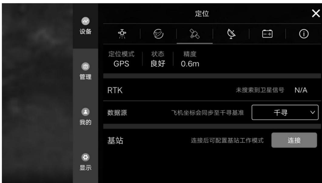
Step3: Click the connection button in the status bar of the base station and select the Bluetooth address of the corresponding RTK base station.
