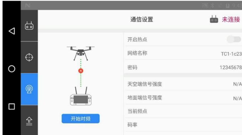
2. Click the "Start Frequency Matching" button, the indicator light of the remote control will be light green flashing. APP shows a pop-up of "frequency matching" and there is a 30s time limit to turn on the remote control. The receiver turns from green flashing to solid green, and the remote control quickly beeps for 4 times to show frequency matching is successful.
