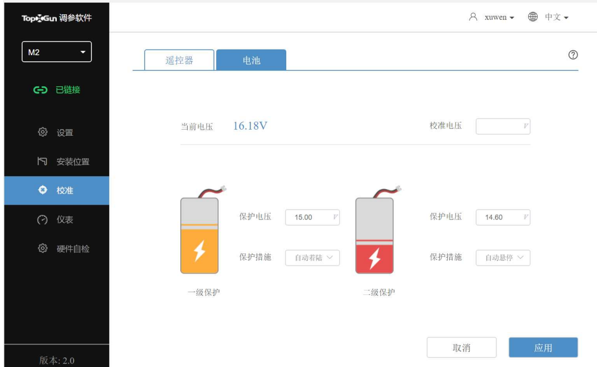
Fig.2-8 voltage protection setting
