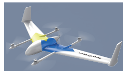
▲ Vertical take-off and landing fixed-wing UAV
